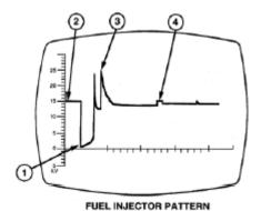
At what point in this scope pattern would the fuel injector be open?
